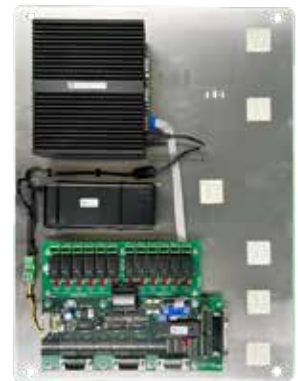
Lane scoring baseplate with scoring computer & I/O interface boards 551122
